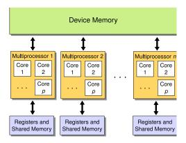
Figure 1: Architecture of a modern NVIDIA graphics card. Figure taken from [20].
